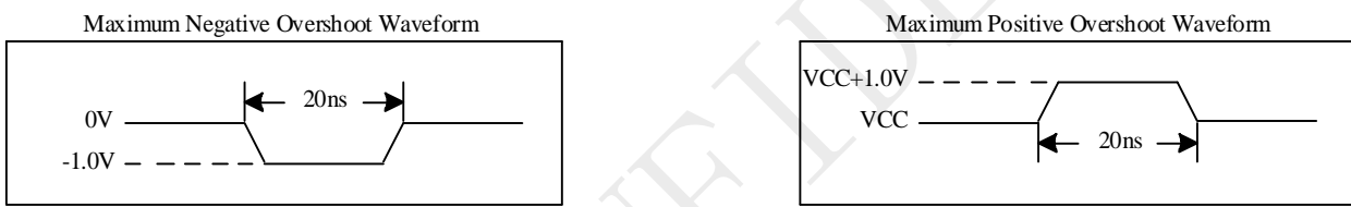
Figure 5-1 Maximum Overshoot Waveform
